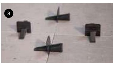
8- Grout joints should be at least 1 mm for interior flooring and 5mm for exterior paving. For installations with offset joints, stagger the tiles at the  $\frac{3}{4}$  point. Self-levelling tile spacers are recommended.
