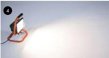
4- The workplace must be adequately lit to detect possible installation defects easily, especially lippage between tiles. Electric site lighting is recommended, to provide brighter than normal light.
